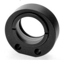
Optical Component Mounts 40CM can be used to hold round thin optical elements of standard sizes. Mounts vary in dimensions so as to support diameters from 10 to 50mm (0.5" to 2"). Original design allows to decrease the mount's dimensions and weight. Mounting holes: one M6 and two Ø4.5 mm. Material: black anodized aluminum.
