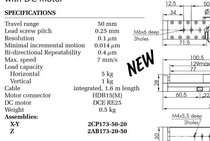
**DC motor** provides **smoother motion** and **closed loop operation**. High number of motor reduction gear provides high resolution, but low speed in turn. Ideal for applications demanding high accuracy but not sensitive to speed limitations.
