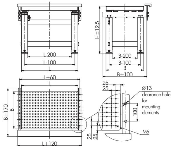
**Laser shelves** are optional breadboards. They save space when installing lasers and other equipment beneath honeycomb table tops. The shelf stays mechanically coupled to the table top.
