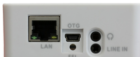
Back view. Left to right: Ethernet connector , mini-USB type B , switch to transfer into FEL mode , earphone and line in connectors .
